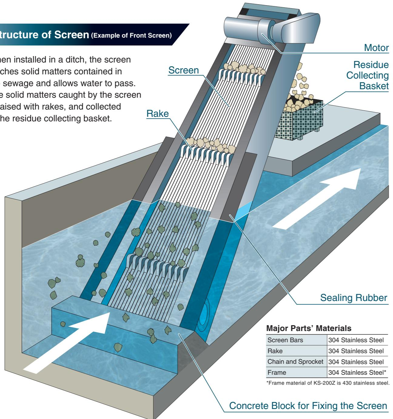
Used for combined sewage treatment tank (Johkasou/septic tank) and small-scale sewage treatment facilities, etc.
