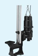
This compact guide rail fitting system is ideal for installing on prefabricated lift stations. Its discharge flange is compatible with major flange standards including ANSI 150lb, BS PN10, and DIN PN10. Four models are available and can be used on Tsurumi cast-iron pumps in the 50 mm through 100 mm discharge bore range.
