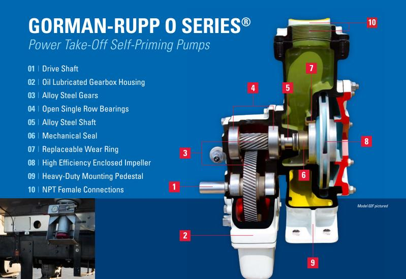
Gorman-Rupp selfpriming centrifugal Power Take-Off Pumps are ideal for handling aircraft fuels, fuel oil, gasoline and other petroleum derivitives.
