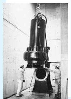
B-series pumps are working in many sewage treatment plants throughout Japan because of their excellent reputations. As durable motor is tough enough against frequent ON/OFF, automatic unattended operation by central control is available.
