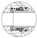
86B3-B SEAL DETAIL Type 21, Mechanical, Self-Lubricated. Carbon Rotating Face. Ni-Resist Stationary Face. Fluorocarbon Elastomers (DuPont Viton® or Equivalent). Stainless Steel No. 18-8 Cage and Spring. Maximum Temperature of Liquid Pumped, 160°F (71°C).\*
