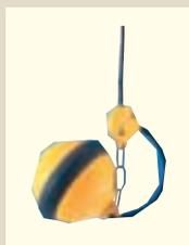
Model RF-5 is an economy type float which can detect upper/lower-limit water levels with single float. The snap on-off action ensures stable operation in clean or waste water containing suspended solids or oil and fat.
