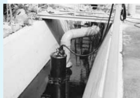
B-series pumps being used for a temporary installation during rainy season. It is used to pump up water of branch river to the main stream when the water level of main stream becomes higher than that of the branch river.
