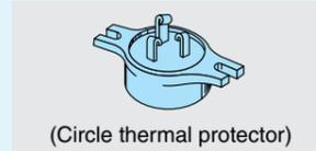
Miniature Thermal Protectors (MTPs) are imbedded in the winding of the pumps of star delta starting. These MTPs are connected in series, and their wires are led out of the motor. Should the winding temperature rise to the actuating temperature, the bimetal strip opens to cause the control panel to shut the power supply.
